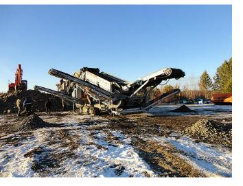
MATERIAL : coal gangue FEEDING SIZE :0-600mm OUTPUT SIZE : 0-30mm CAPACITY (TPH) : 100-150T/h EQUIPMENT : YG938E69mobile crushing station、 Y3S1860CS160mobile crushing station、B800×10m Belt conveyor
