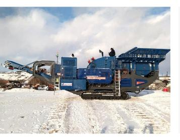
MATERIAL : coal gangue FEEDING SIZE : max. 600mm, most 450mm OUTPUT SIZE : 0-50mm CAPACITY (TPH) : 220T/h EQUIPMENT : PF1315 impact crusher、 PFP1315 Crawler Mobile Crusher
